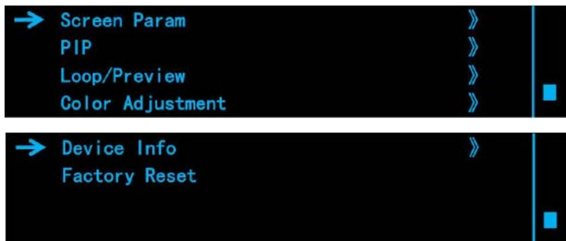
Screen Param: Same with Scale, to adjust screen size
