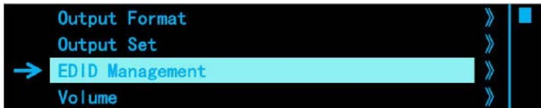
Press EDID input interface by knob (The adjustable interface can be revised).
